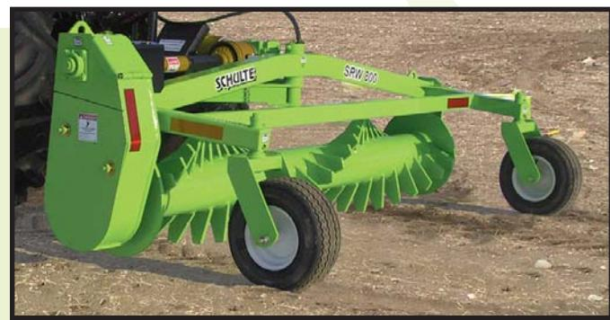
Check out Schulte's high quality conveyor type and reel type rock pickers. These machines are your best choice for continuous picking of windrowed rocks.
